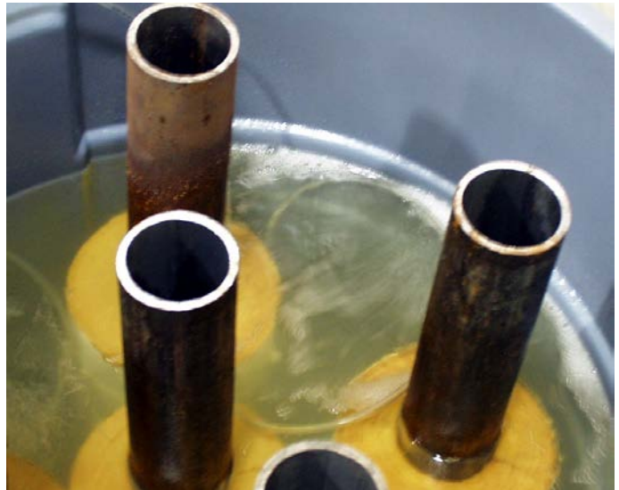
Reactive Gel coated pipes in 5% salt water
