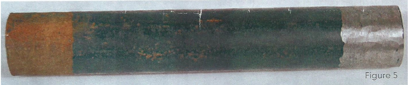
Pipe treated with Petroleum Hydrocarbons with Thickeners on one end. Then exposed to the Florida costal elements for one month
