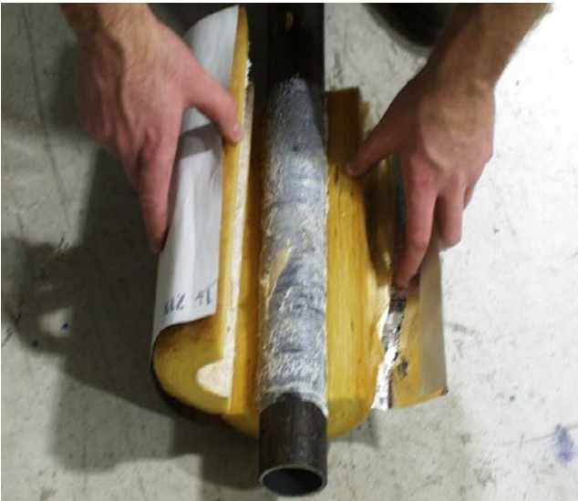
Reactive Gel Applied to Pipe
