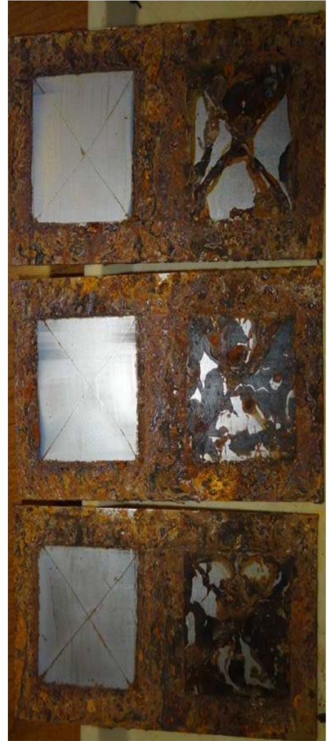
Post Exposure – After Coating Removal
