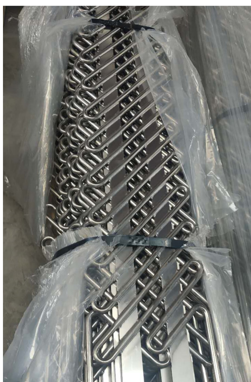
In the static mixer reactor, the adhesive passes through the unit's shell while the heat transfer medium flows inside a fixed-tube geometry that provides a static mixing effect for uniform and efficient heating and mixing.
